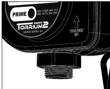
For pumps with a 1" male outlet (e.g. XP350, XP450, XJ50, XJ70 and XJ90) a adaptor socket (P/No. 44992) is required. Thread sealing tape will be needed when using this adaptor socket to ensure a watertight seal.
